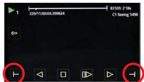
Play Cine files in RAM. Tap forward or reverse multiple times to speed up playback. Tap in and out points and save to CineFlash. Apply a long press over the in & out markers to reset
