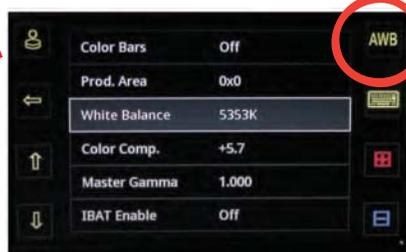
The camera's white balance can be set with the AWB on the upper right or manually by adjusting the color temperature and color compensation
