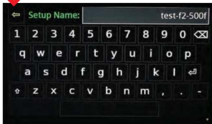
When saving a user-setup, enter a name and tap the 'return' button to save it. Any of the 3 factory-saved presets can be modified or overwritten
