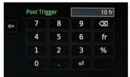
The Post Trigger can be entered in frame count or percentage. The value represents the amount of frames past the trigger point to be stored in RAM
