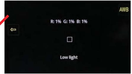
AWB automatically adjusts the camera's white balance. Place a white or neutral object in the center square and tap once. White subject must not be fully saturated
